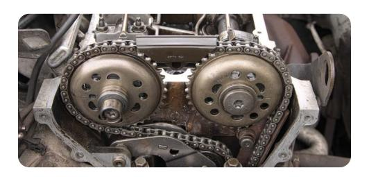
To combat the issue of soot, the industry developed the Sequence X Engine Test (ASTM D8279) specifically to measure an oil's ability to resist soot and fight timing-chain stretch. It's part of the API SP and ILSAC GF-6 motor oil specifications introduced in May 2020 and the latest API SP and ILSAC GF-7 specifications released in March 2025.
